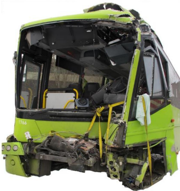
Figure 5: Damage to the front of the westbound bus. Photo: AIBN
